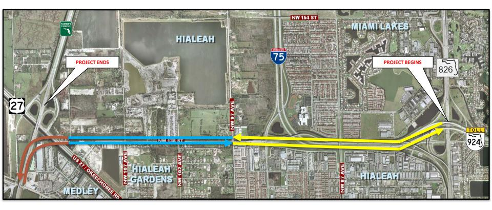
Two-lane ramps to and from the south only, will connect Florida's Turnpike with the NW 138<sup>th</sup> Street corridor providing a direct connection west of NW 107<sup>th</sup> Avenue.
